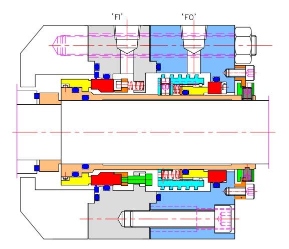
90 SERIES MULTI SPRINGS MECHANICAL SEAL TYPE 9602/9101 DOUBLE MECHANICAL SEAL ARRANGEMENT WITH DIFFERENT API PLAN 53
